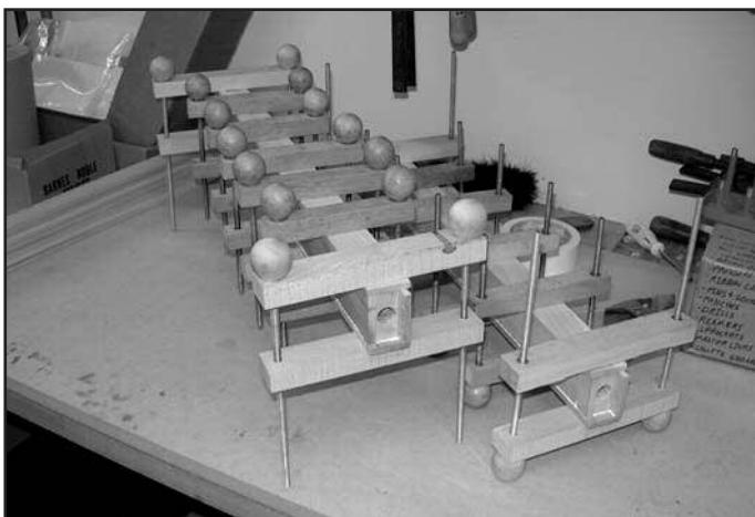
Figure 14. Fronts glued and clamped to pipe body.
