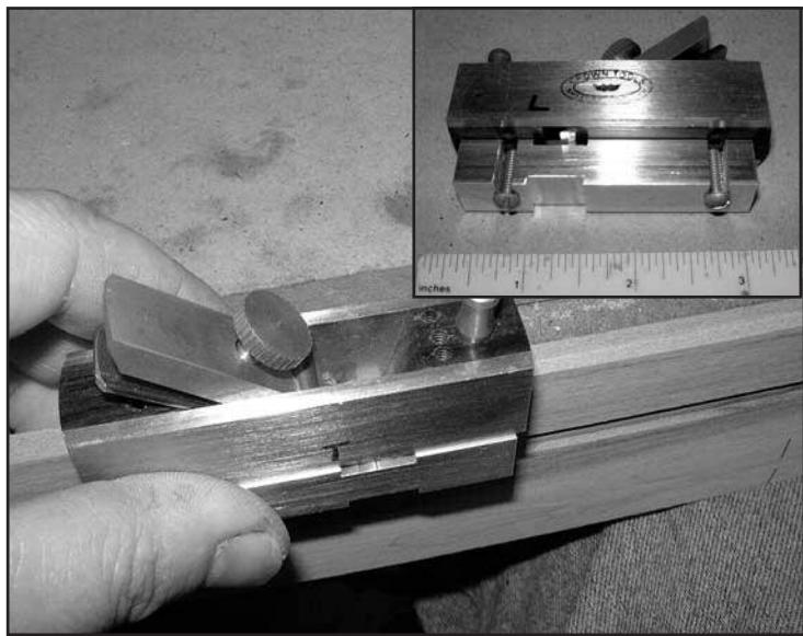
Figure 8 & 9 (inset). Miniature hand plane set up (above); below it is seen being used to cut the tuner groove.
