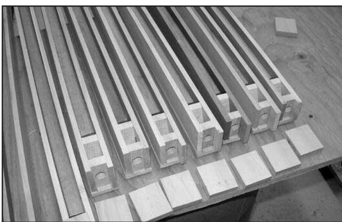
Figure 15. Pipe bodies before fronts are glued on. The windways are machined to depth, and material prepared for caps.
