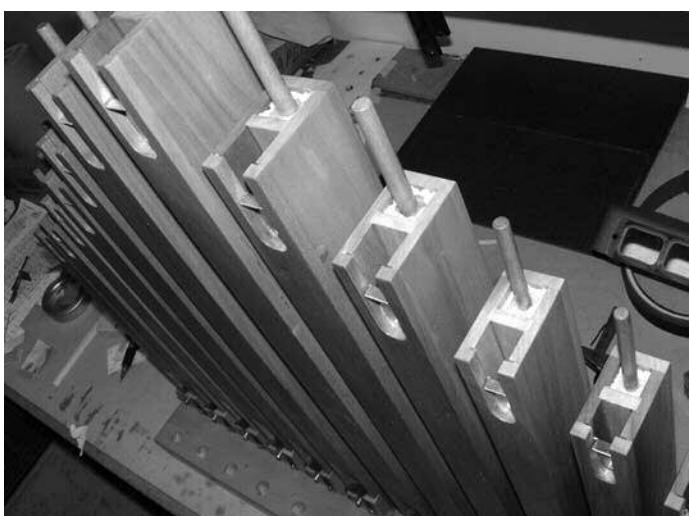
Figure 23. Finished pipes with stoppers and tuners in place. The front and back chambers of these pipes are clearly visible.
