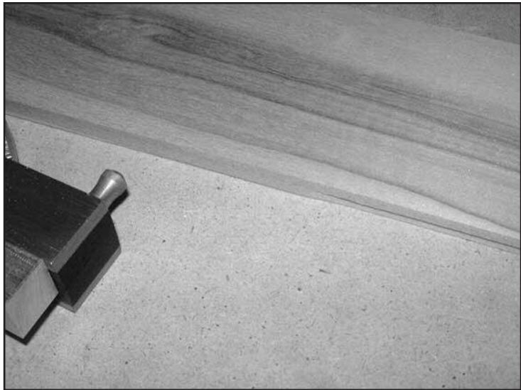
Figure 7. Pipe side with tuner groove, and center groove for center divider.
