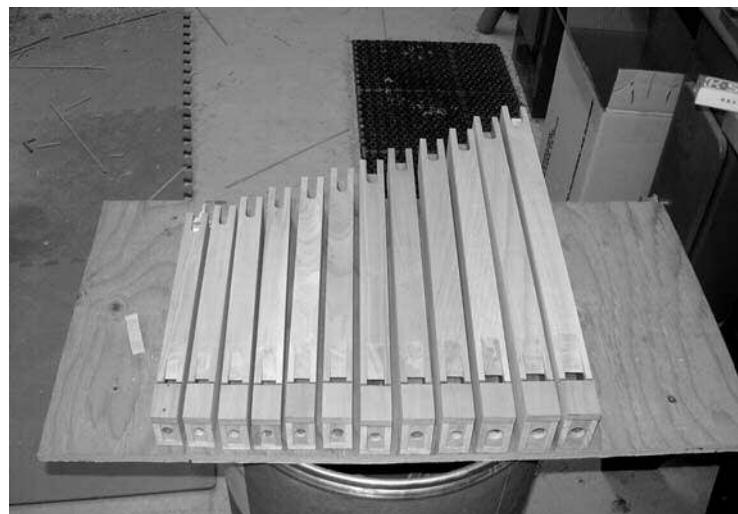
Figure 17. All pipes finished to length, and sides machined flush with the sides.
