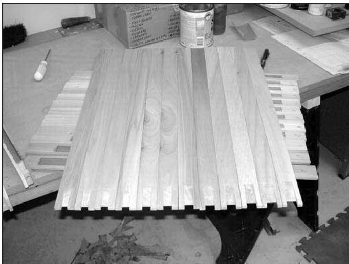
Figure 13. Pipes fronts with upper lips finished.
