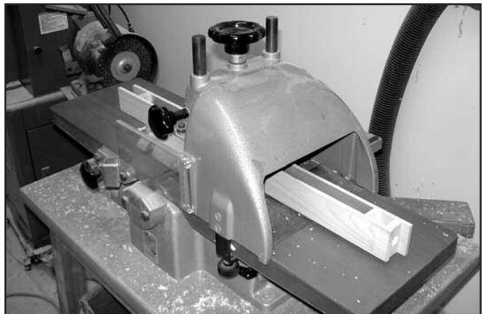
Figure 11. Pipe being machined to proper depth with thickness planer.
