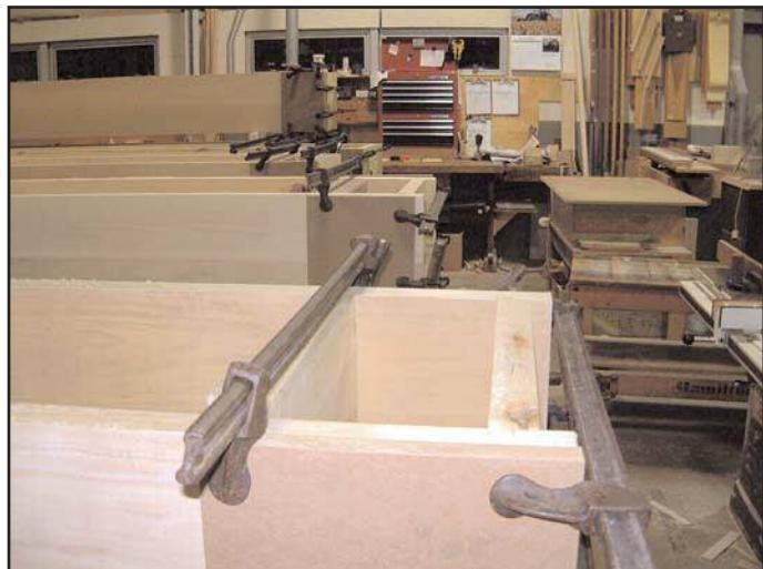
Figure 2. Haskell bass pipes being glued up at O.S.I.
