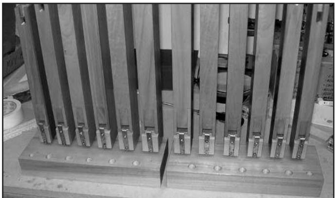
Figure 22. New left and right toe board with accompaniment Haskell violin pipes in place.
