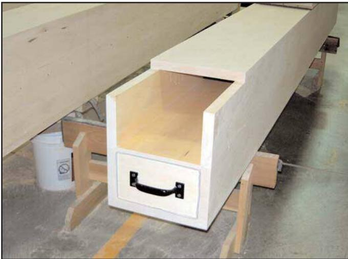
Figure 3. Open end of Haskell bass pipe. The back chamber is adjustable by means of a stopper.
