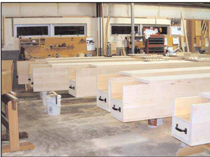
Figure 4. Partial set of Haskell bass pipes; stopper handles are visible.
